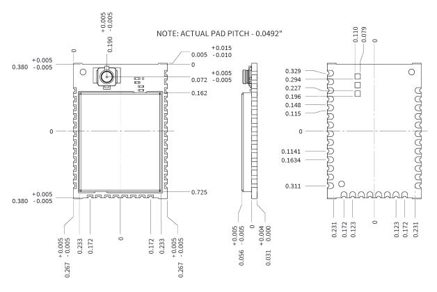
Mechanical drawings XBee3 micro antennas
